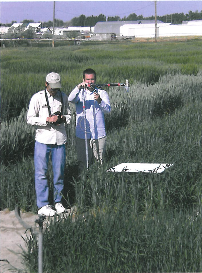
UI Ph.D students Junli Zhang (L) and Brian Bowman (R) use Canopy Spectral Reflectance (CSR) to evaluate grain yield, water use and nitrogen use efficiency in different wheat lines at the Aberdeen Research Center.
