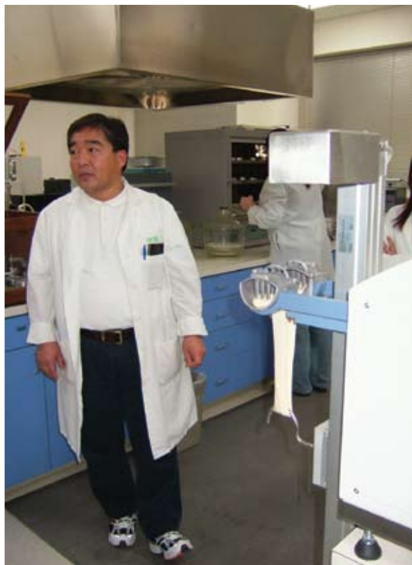
Bon Lee from the Wheat Marketing Center, demonstrates how the Extensigraph measures dough extensibility. The resistance to extension accurately predicts the suitability of the dough for use in various products.
