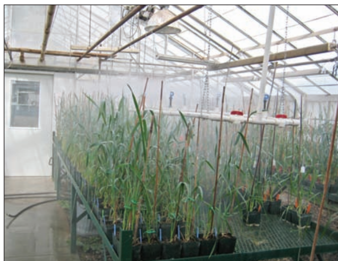
Misting mimics the field conditions of high humidity and warm temperatures necessary for infection of wheat by Fusarium species causing Fusarium Head Blight.
