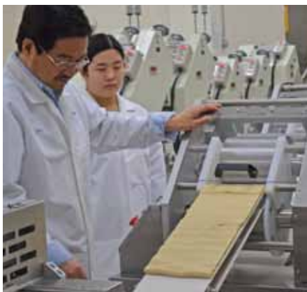
Laminating cracker dough on the pilot line.
