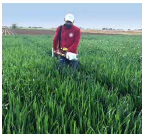
Arjun Pandey, reading plant stress in winter wheat plots using the GreenSeeker remote sensing instrument.
