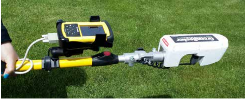
Close up of the hand-held GreenSeeker remote sensing instrument.
