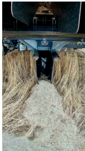
Simple chute for placing chaff in narrow line. Photo by Claudio Rubione.
