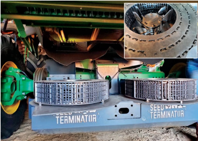
Weed seed mill on combine. Inset shows a top view of the mill.
