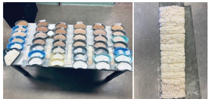
Large flour slick (right) highlights visual differences of every step in the reduction process.
